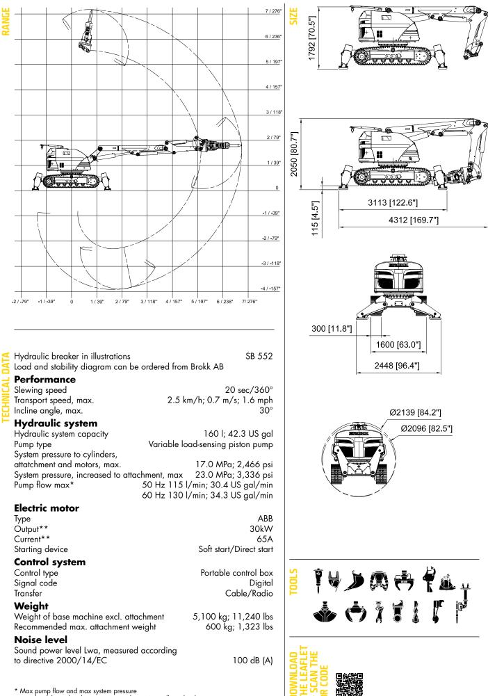
\* Max pump flow and max system pressure cannot be delivered at the same time as the engine will overload
