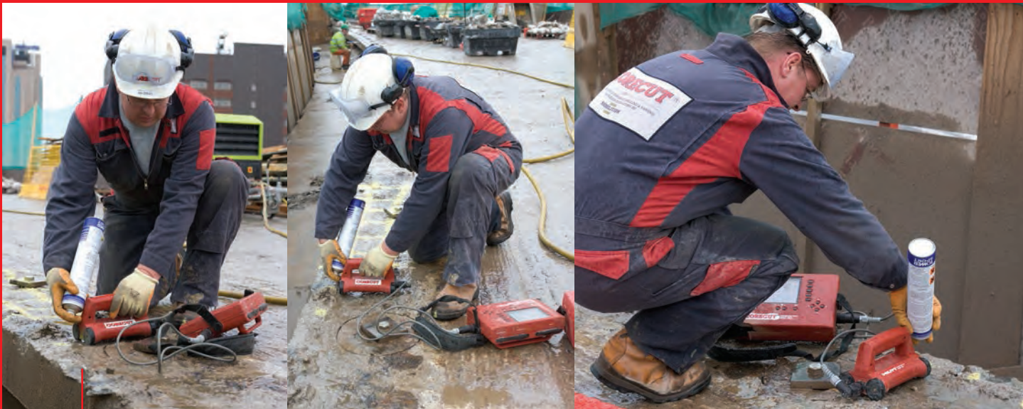
Reinforcement Survey to Bridge Deck
