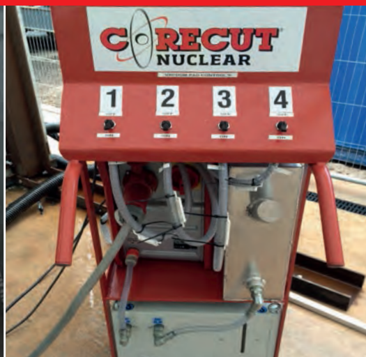
PROSHAVE 210 vacuum pad and Cooler Control Console
