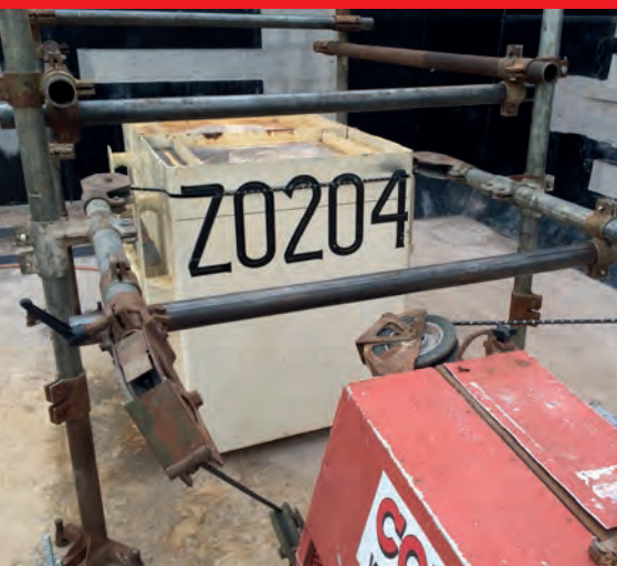
Size reduction of steel skip at our In-House trial facility
