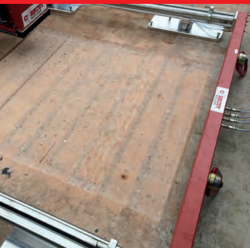
PROSHAVE 210 Electric System fixed using vacuum pads
